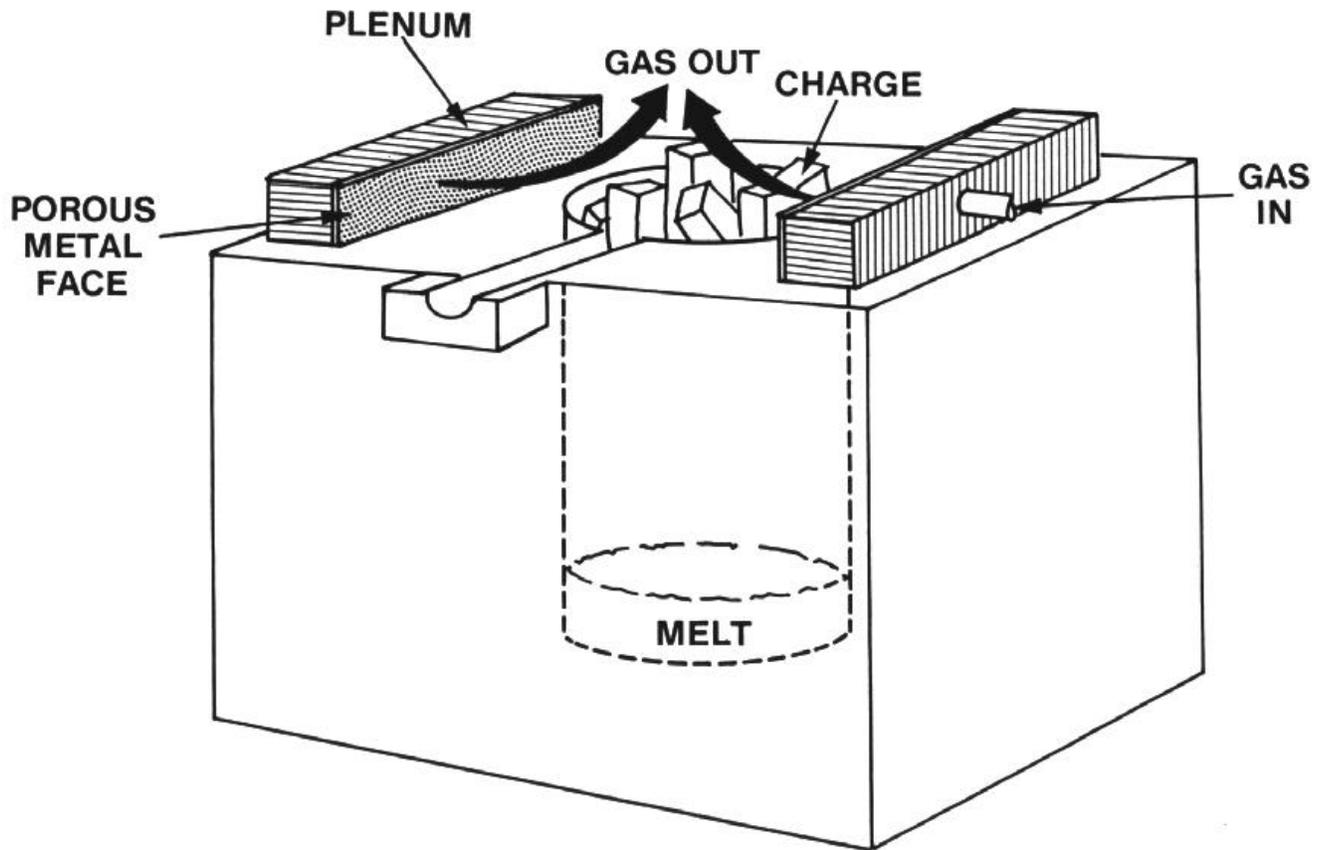
Figure 1: Schematic of Laminar Barrier Inerting on an Induction Furnace
