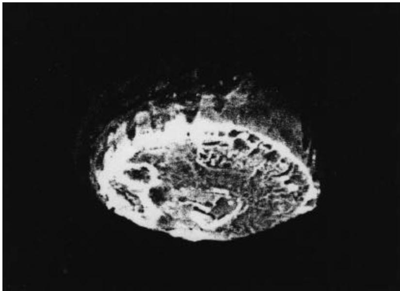
**Figure 3: Slag Formation in Air-Melted Heats**
