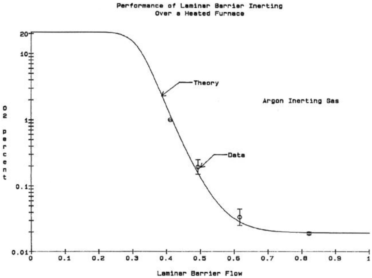
**Figure 2: Headspace Oxygen Content as a Function of Laminar Barrier Flow.**
