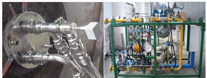
**Fig. 4. DOC-JL burner and oxy-fuel control system valve rack**
