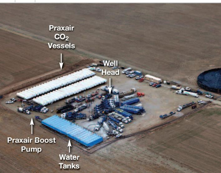
*Solubility and Viscosity* – Used extensively since 1962 as an additive to acid fracturing, CO<sub>2</sub> is very soluble with oil and water. Due to its solubility, it greatly reduces viscosity (especially of oil) during a fracturing treatment.
