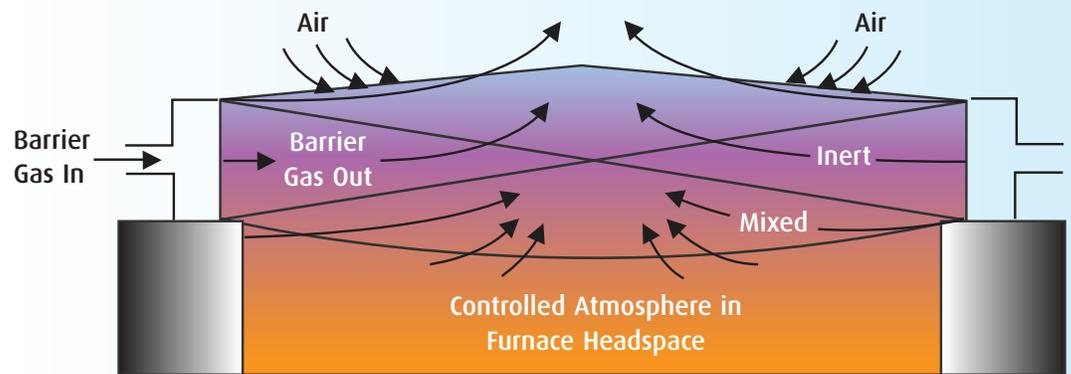
*The wide laminar barrier issues from the porous face of the plenum and flows across the furnace opening. Close to the furnace opening, some of the controlled atmosphere from the head space mixes with the barrier gas. Above the laminar barrier flow, a small amount of air mixes with the barrier gas, but essentially no air is allowed to pass through the barrier and into the furnace.*
