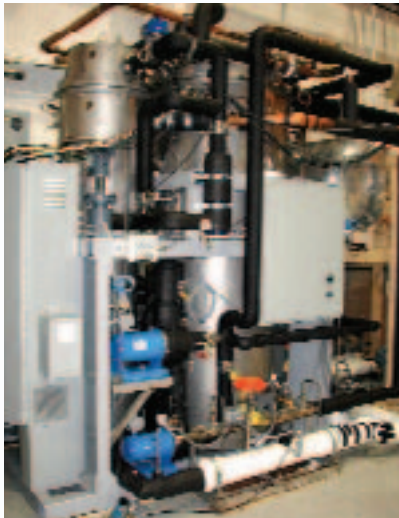
Praxair's NCOOL system employs proprietary, patented buffering technologies that minimize freezing during heat exchange between the cryogenic liquid nitrogen and the process fluid or cooling media.
